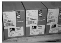
Compliance requirements also are useful within a manufacturer's own facility. Bar codes on compliance labels identify the product serial number and other important product information. Bar code scanners or data collection terminals read this information and communicate with a computer host that processes the data. Bar code scanning improves the accuracy and the timeliness of the data.
