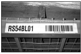
A warehouse operator transfers the material to an inventory location. These sites often are identified with bar codes printed on reflective labels. The reflective material (such as Zebra's RetroScan 4000 labels) improves readability from fork trucks up to 30 feet away. Bar codes are necessary because the operator scans both the package and the new storage location to complete the transfer operation and record it in the system.
